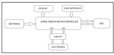
An analog-to-digital converter is used to measure the small nanoampere to microampere range current that results between the counter and working electrode. With the presence of a contaminant in the medium, the interaction between the contaminant and the DNA on the electrodes produces a deviation from the base current-potential relationship, which can be related to the concentration of the contaminant. The microcontroller is then used to analyze the data and display results.
